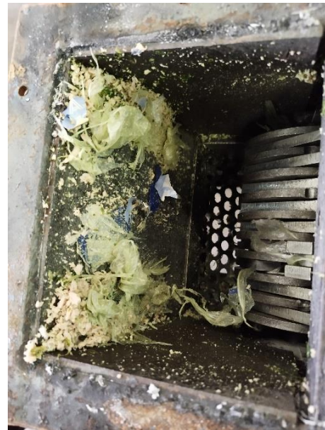
Figure 2. Test comminution in a hammer crusher.
